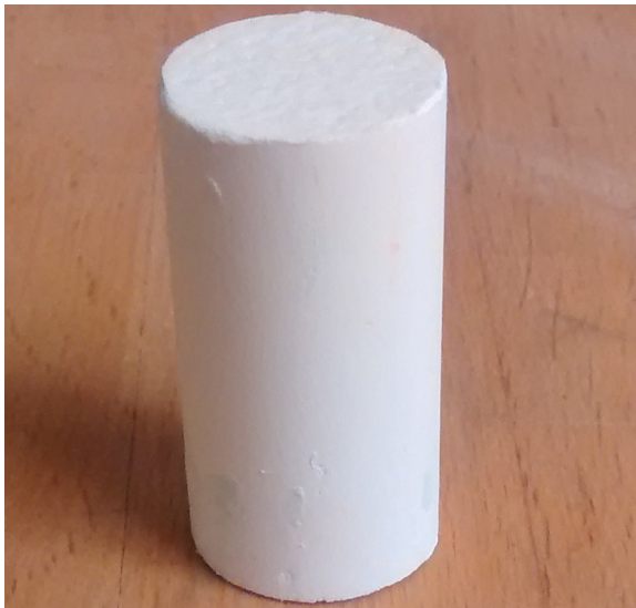
CaCO 3 cement specimen (20 mm dia., 40 mm height) with initial mixture design ACC:V 1:1 wt. %.
