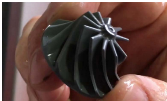
Figure 13. High resolution silicon nitride structures produced by vat photopolymerisation
