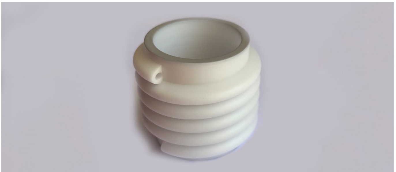
Figure 10. A concept power tube with an integrated cooling channel printed in Morgan AL-300™ grade alumina and metallised to allow for joining with other parts, forming a vacuum tight assembly.
