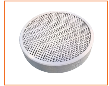
Lattice filter structure engineered to improve performance [Source: MTC]
