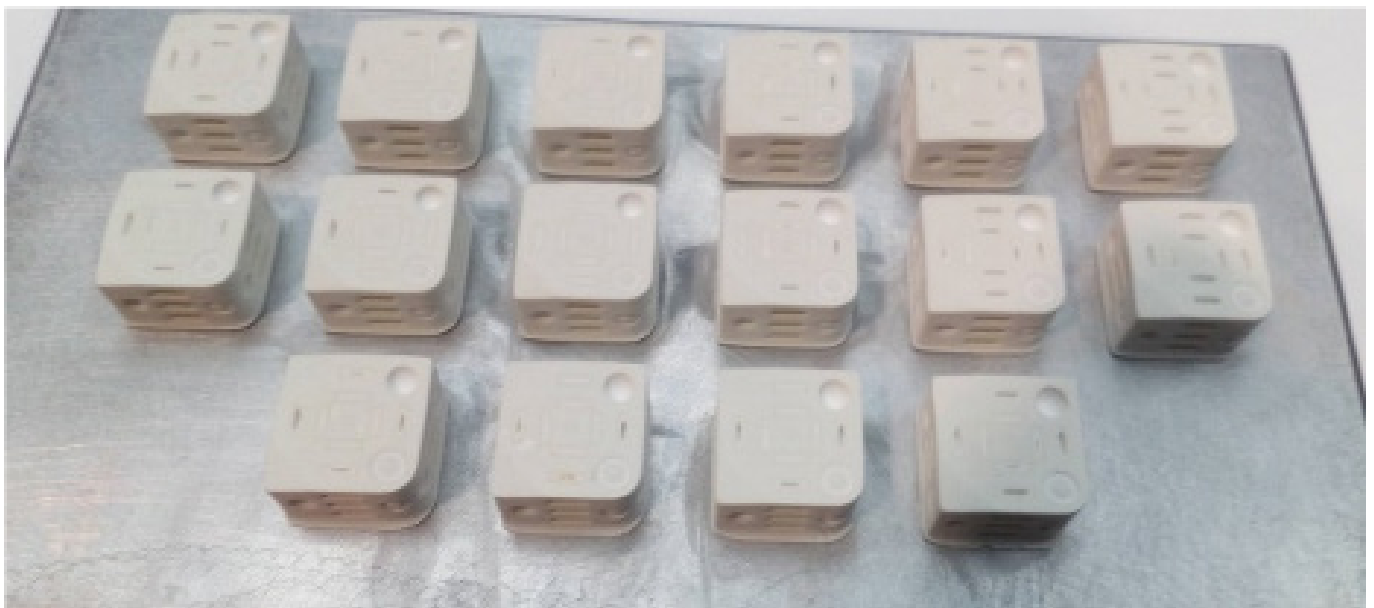
Figure 5. Simple test cubes for evaluation of process variation across print bed
