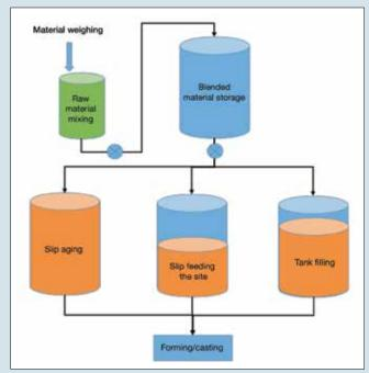
Figure 2. Schematic of typical three-tank slip storage system often utilized within clay-based production systems.
