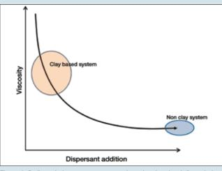
Figure 3. Deflocculation curve representation, showing the deflocculation level utilized for clay and non-clay slip in relation to the viscosity of the associated suspension.
