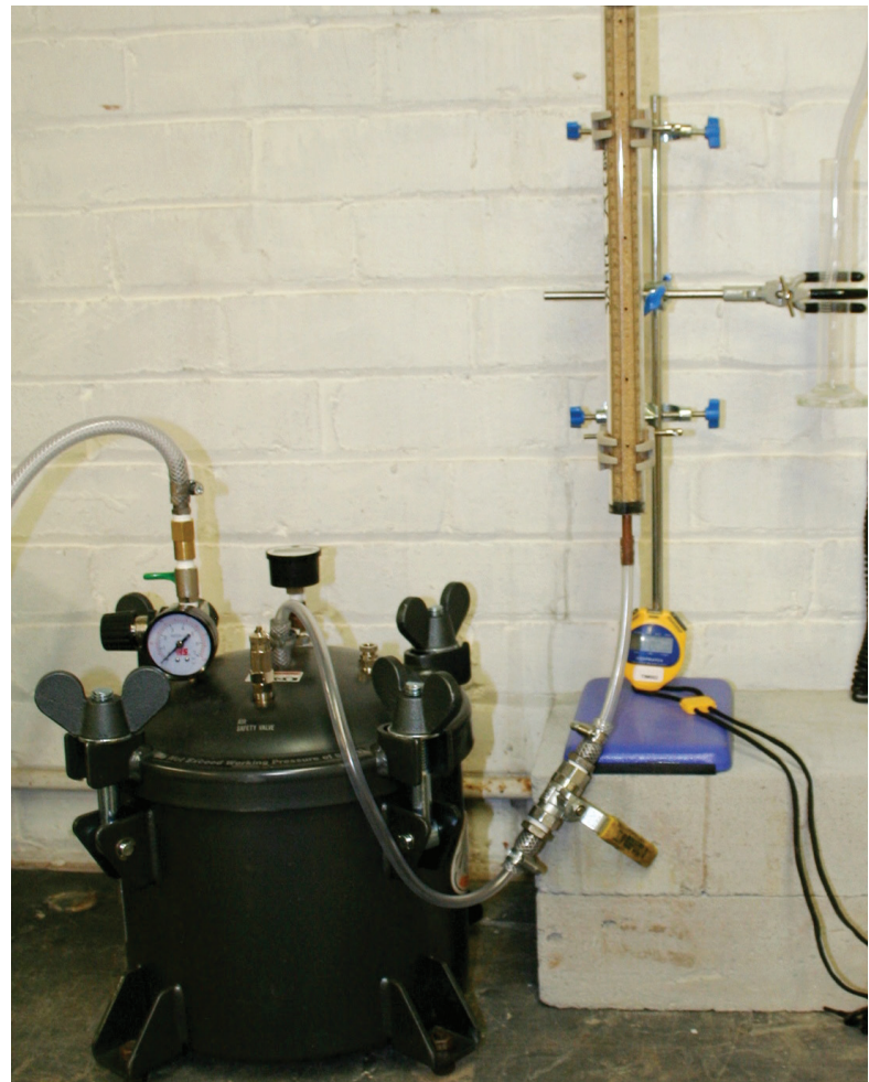
Figure 4: Column test (damp) showing sample progressing through the column.
