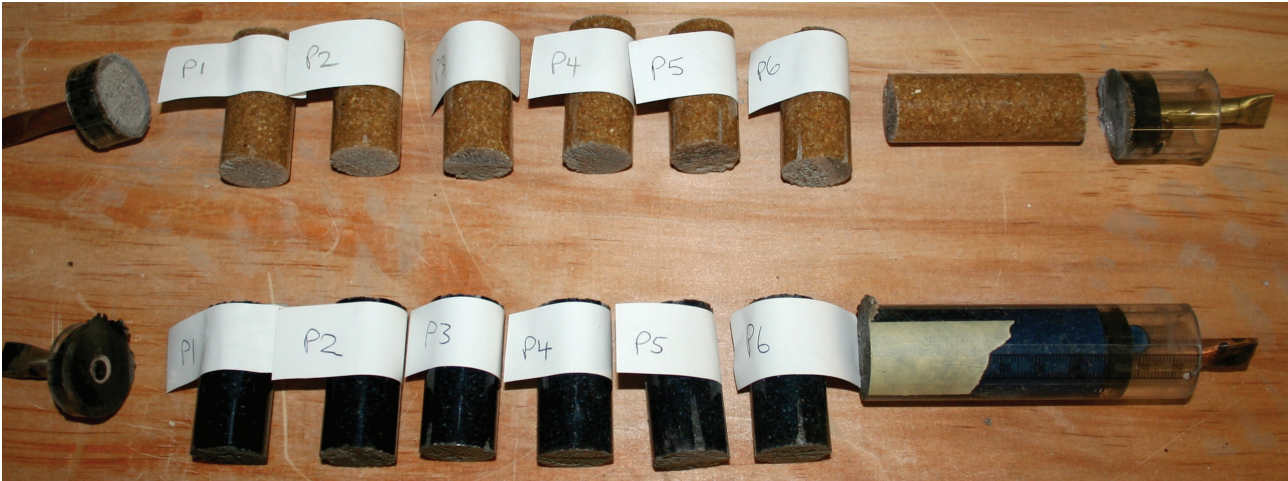
Figure 5: Six cylindrical samples from two test columns.
